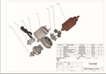
A starter motor is used to rotate an engine to begin the combustion process. A flex plate or flywheel is connected (bolted) to the rear of the crankshaft, these unit are fitted with a ring gear which anables the starter to be activated if the flywheel is worn it can cause a grinding noise when the starter is operated.
